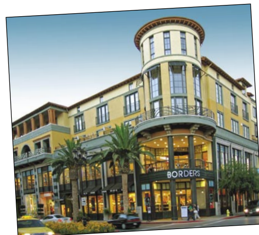
Mixed-use development can combine retail or commercial at the street level with residential or office above
